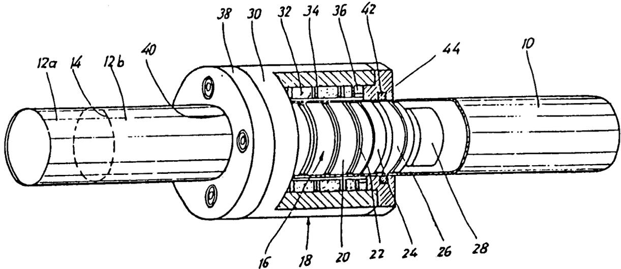
Inside the cylinder, the piston is driven by a pressurized fluid. Stoll patent, col. 3, ll. 13-19. As the piston travels through the cylinder, the magnetically coupled sleeve follows the piston along the outside of the cylinder. Id.
